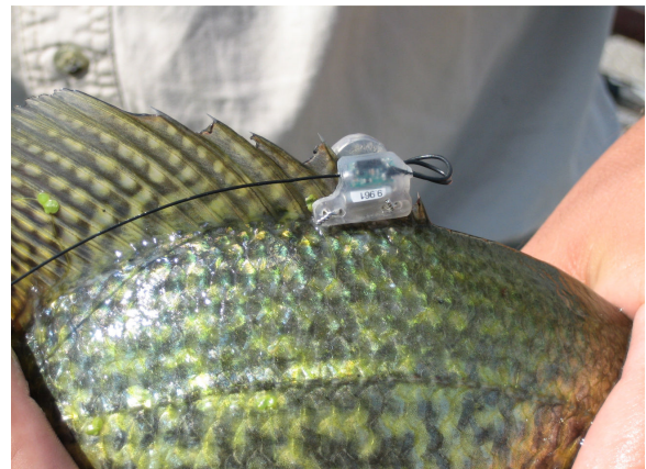
Figure 3. Photo showing attachment of experimental transmitter to the dorsal spines of a black crappie in Pool 11, Upper Mississippi River.
