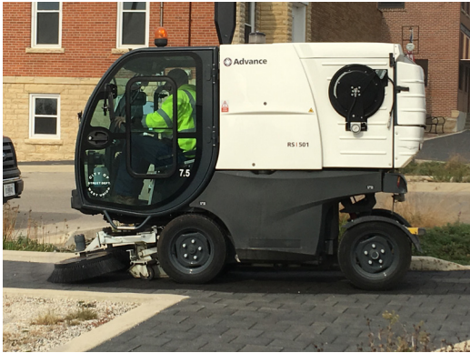
FIGURE C8-S3-1: Mechanical sweeper sweeping PP
