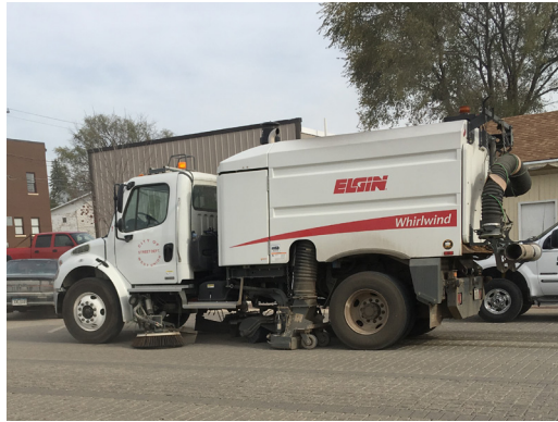
FIGURE C8-S3-2: Regenerative air cleaner cleaning PP
