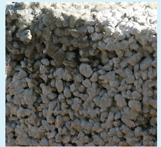
FIGURE C8-S1-4: Pervious concrete examples.
