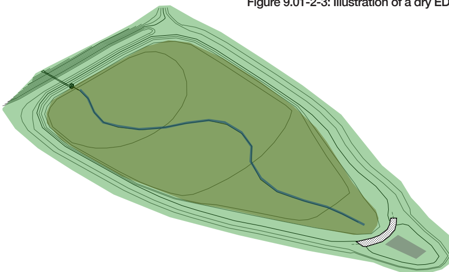
Figure 9.01-2-3: Illustration of a dry ED detention basin
