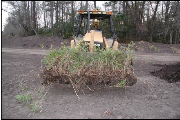
Photo 31. Sod mat harvest with a front-end loader. Source: Buck Engineering
