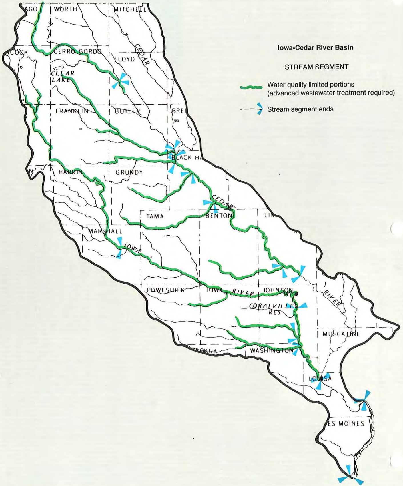
FIGURE 4-1 Stream Reaches Where Advanced Waste Treatment Will be Required: Iowa-Cedar River Basin
