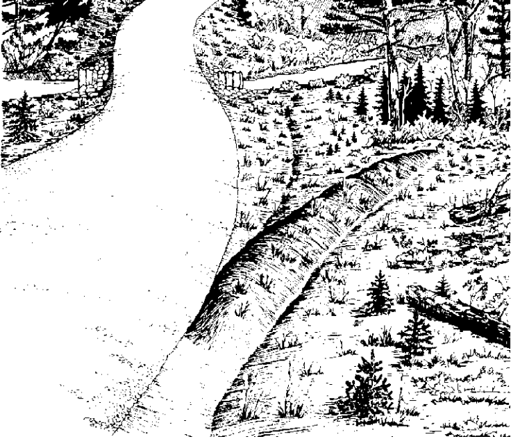
Figure C-2. Diversion ditch. (Adapted from Wisconsin Department of Natural Resources, 1995.)
