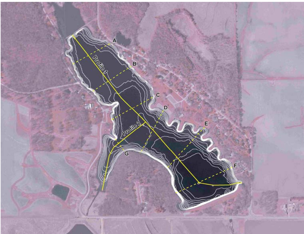
Figure D12 Union Grove Lake showing profile and cross-section alignments
