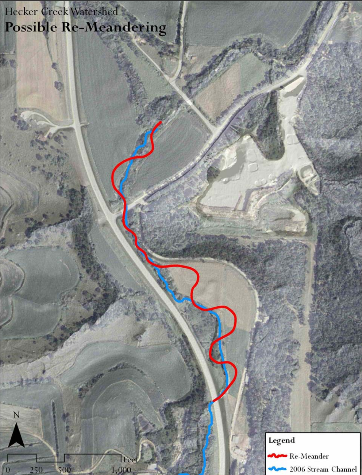
Figure 6-1. Rough sketch of possible re-meandering of channel in lower portion of Hecker Creek. (Provided only as an example, not based on stream restoration guidelines.)
