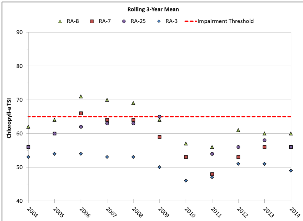
Figure 3-4. Rolling 3-year mean Chl-a TSI for Rathbun Lake segments. Green triangles – S. Fork Chariton arm of the lake (Site RA-8, Segment IA 05-CHA-0020-L_2); red squares – Chariton arm of the lake (Site RA-7, Segment IA 05-CHA-0020-L_3); purple circles – Honey Creek arm (Site RA-25, Segment IA 05-CHA-0020-L_4, and blue diamonds – main body near dam (Site RA-3, Segment IA-05-CHA-0020-L_4). Red-dashed line illustrates the impairment TSI threshold value of 65.
