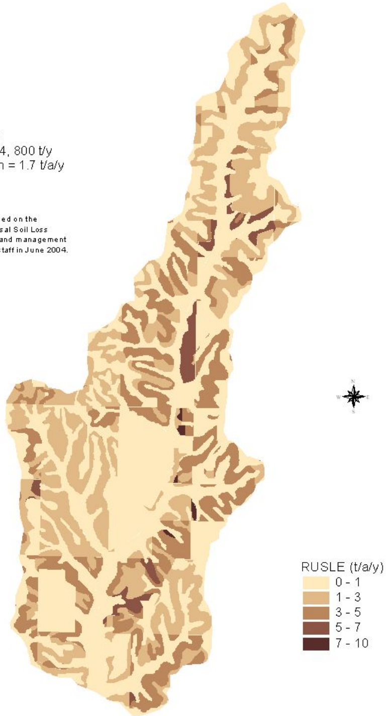
Figure C-1. Sheet and rill erosion as in the watershed of Pierce Creek Lake.
