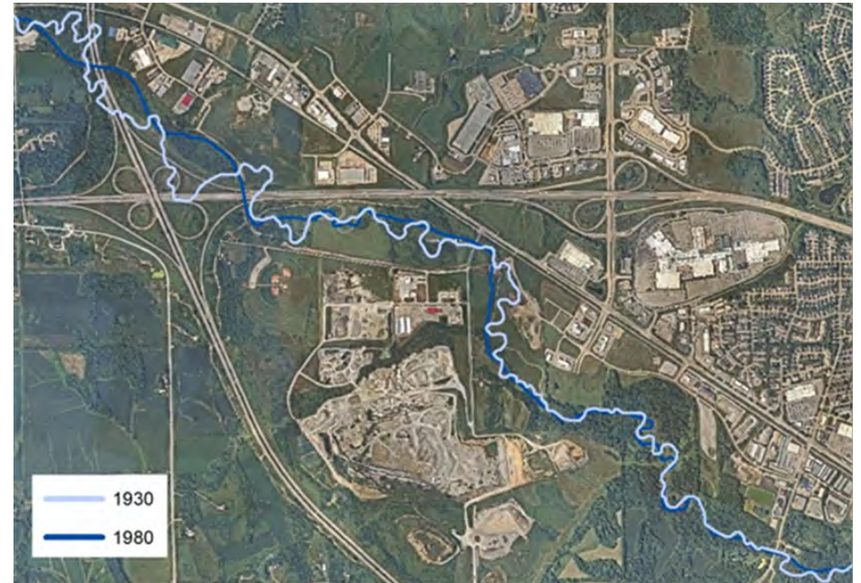
Figure 4-9. Clear Creek Centerlines in 1930 & 1980 with 2017 Aerial Imagery
