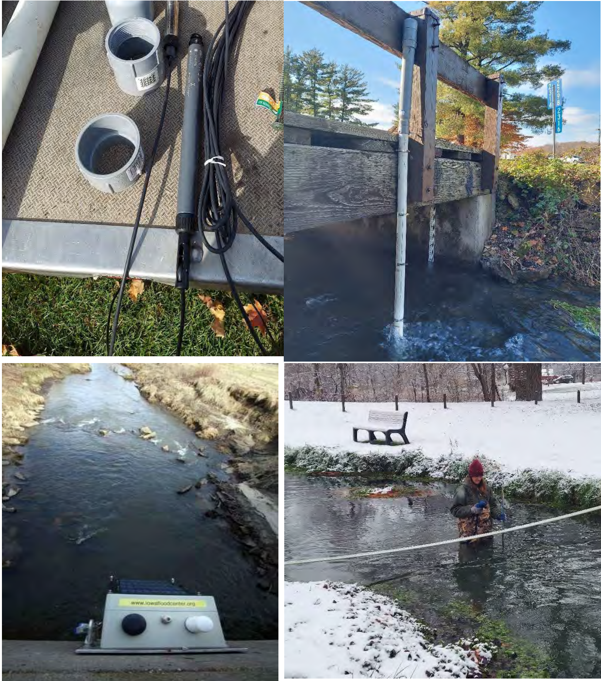
Figure 51. Upper Left and Right: Stream stage sensor installed below Siewers Spring. Lower Left: Stream sensor installed on bridges in Trout Run. Lower Right: measuring flow of Siewers Spring to establish a stage-discharge relationship.
