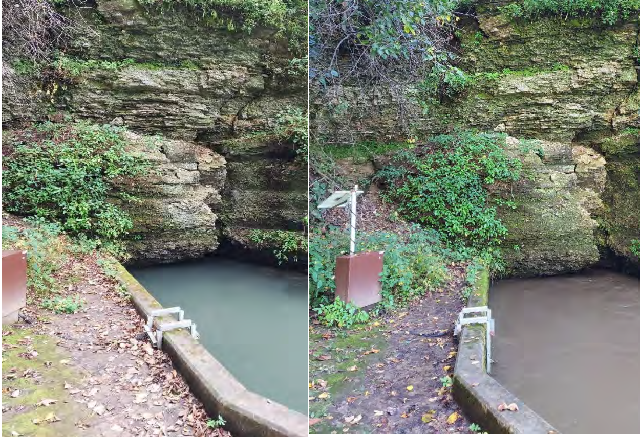
Figure 10. Differences in Siewers Spring water clarity (i.e. turbidity). Left: Siewers Spring turbidity is 6.9 NTU and increases to 45.9 NTU (right) after a rain event in the Trout Run Watershed.
