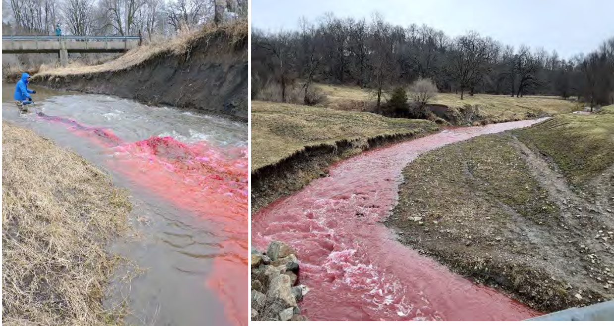
Figure 43. Left: Rhodamine dye poured into Trout Creek above a losing stream segment in Nordness. Right: Trout Creek surface waters one mile below dye input location.
