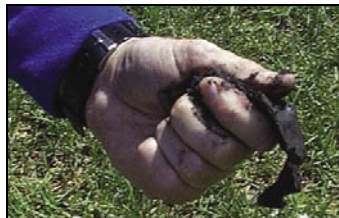
Ribbon test used to estimate clay content.
