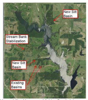
the lake. Finally, approximately 1,200 feet of degraded streambank will be stabilized by re-establishing flood plain benches, rock armoring supplemented with the planting of live stakes, installation of rock riffles, and the installation of stream bottom vanes constructed from salvaged logs. The lake will be partially lowered to facilitate shoreline armoring and habitat placement, however boat access will be maintained at the main boat ramp.
