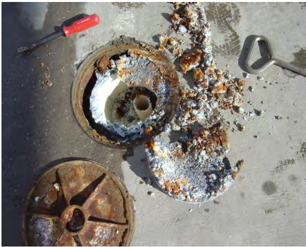
Examples of damaged monitoring wells that are at risk of being conduits for contaminants to the subsurface.
