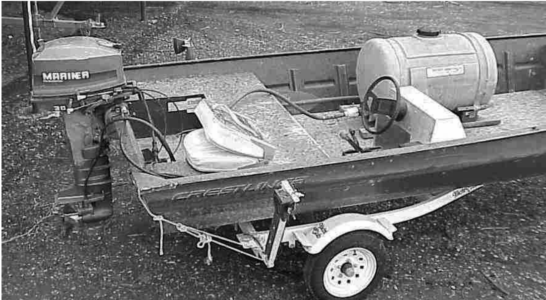
Figure 23. System for liquid rotenone application using a Venturi system on small boat with outboard motor. Note mixing tank for diluted formulation.
