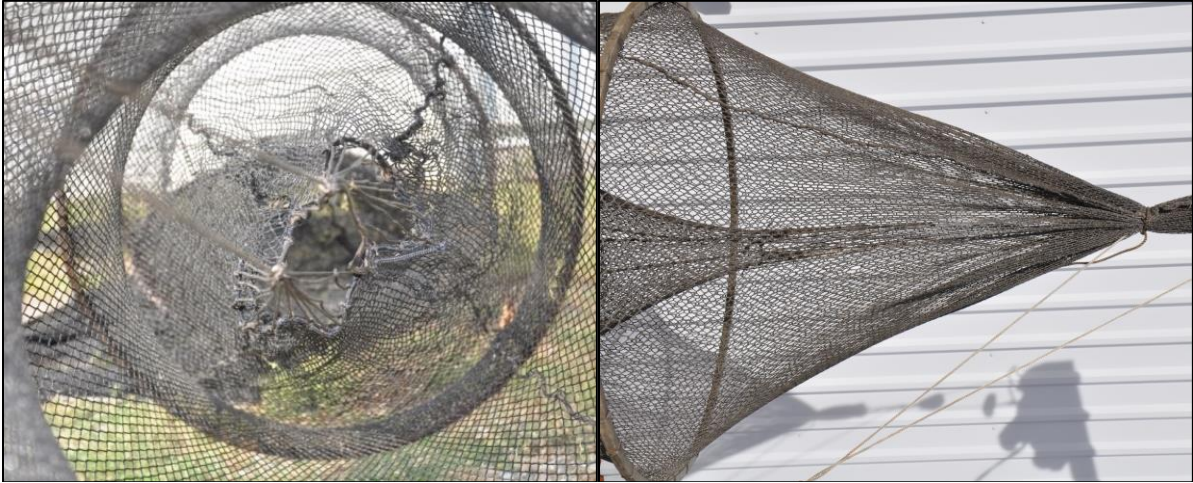
Figure 1. A square throat (A) and a restricted throat (B) on a modified fyke net.
