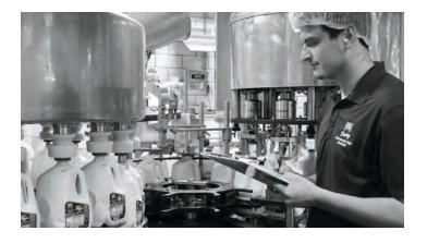
By testing the total solids and butterfat of the product at each purge cycle, it was determined that the product purge cycles can be reduced by at least one cycle, reducing the amount of milk loss generated by this process. The plant is in the process of implementing a one cycle reduction. Further testing on subsequent reductions will be required before full implementation can occur.
