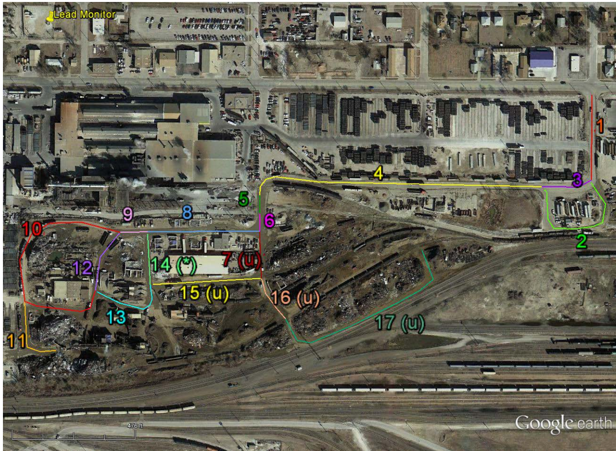
Figure D-1. Depiction of all facility road segments as they existed in the 2010 baseline. (Google Earth's Imagery Date of 3/7/2012.) Unpaved routes are depicted with a "u" and segment 14(*) was originally paved but treated as an unpaved road in the baseline due to surface deterioration.
