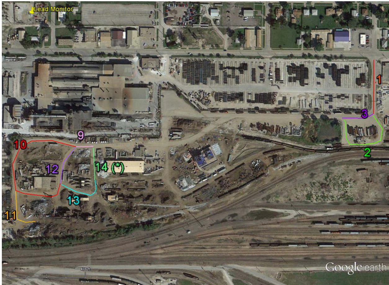
Figure D-3. Road segments whose dimensions and locations are not affected by the addition of the ZC Plant (they are the same as in the baseyear). (Google Earth's Imagery Date of 9/21/2013.) (Note, segment 14(*) is treated as an unpaved road in the baseline and as a paved road in the control strategy.)
