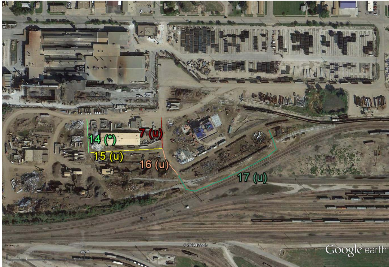
Figure 5-2. Approximate location of the unpaved road segments in the 2010 baseyear at Alter Metal Recycling. Segment 14 was originally paved but was treated as unpaved due to surface deterioration.
